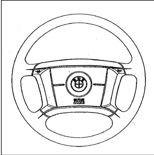
**Airbag-Lenkrad, d = 385 mm >(1)**
